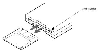
Figure 4-2 Loading/Ejecting a 3.5" Floppy Disk
